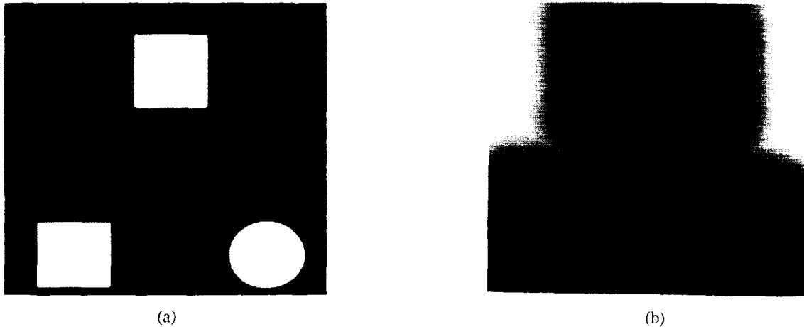
Figure 4 - (a) Three regions for distance computation. (b) Euclidean distance to nearest region.
