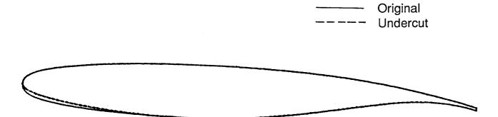
Figure 31. Sketches of 12-percent-thick supercritical airfoil with and without forward lower-surface undercutting.
