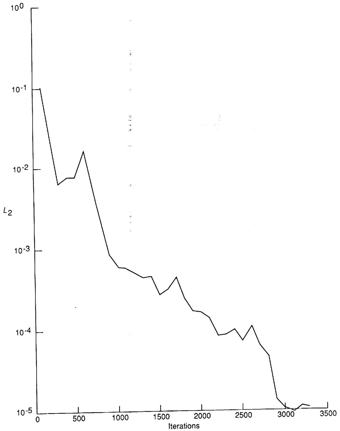
Figure 28. Convergence history for \alpha = -5^\circ and \epsilon_0 = 0.2 on fine grid in domain 1 with C_N \geq 5.0 .
