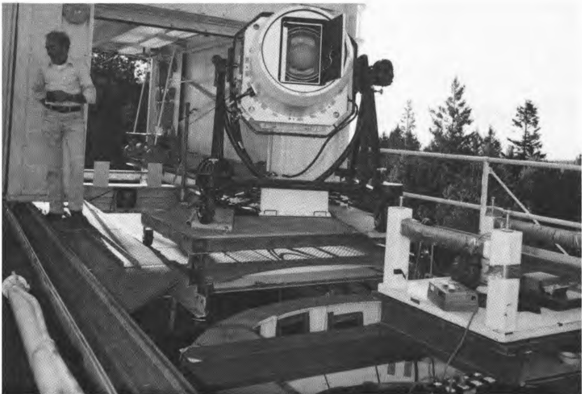
Figure A-12.- LFC in position at the NOAA facility at Cloudcroft. Camera team await darkness and the rise of the moon in preparation for multiple exposures of the lunar disc at various field positions throughout the image format (NASA photo S82-36045).
