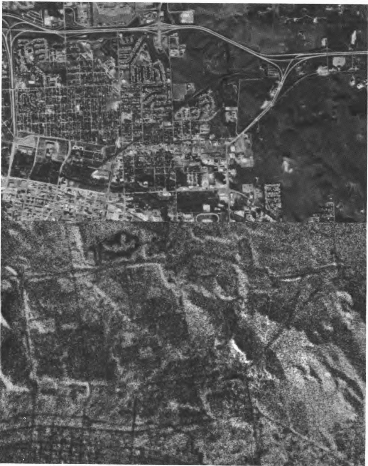
Figure 3-45.- Comparative frames of LFC and MC imagery. LFC frame 1953 (top) and MC 01-0929-32 (bottom) show Rapid City, South Dakota. Shown at same magnification, approximately 20X original size.
