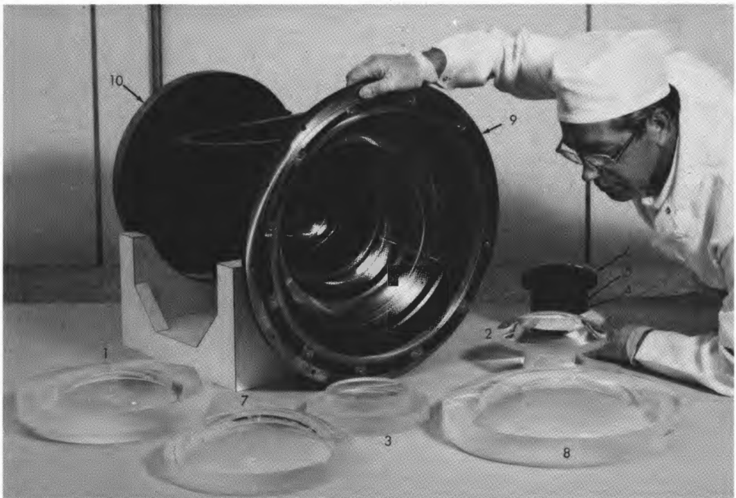
Figure 1-5.- Finished LFC lens components prior to assembly. Shown are the front lens (element 1), the doublet (elements 2 and 3), the triplet (elements 4, 5, and 6), the rear lens (element 8), and the machined lens cell castings (9 and 10). (NASA photo S79-35862.)
