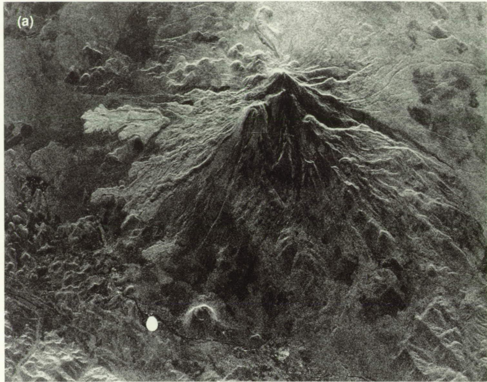
Figure 29. SIR-B images of Mount Shasta at look angles of (a) 28 deg, (b) 51 deg, and (c) 57 deg, corresponding to expected Magellan data from mid- to high and equatorial latitudes of Venus. Geometric distortion increases with decreasing look angle. Most lava flows and domes are detectable on all three images. (d) Generalized geologic map of Mount Shasta (modified from Wagner and Saucedo, 1987).
