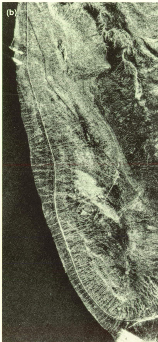
Figure 52. Durmid Hills east of the Salton Sea (Figure 49, box 3): (a) Seasat SAR image obtained at 23.5-cm wavelength in August, 1978; (b) corresponding airborne radar image obtained at 2.4-cm wavelength in November 1985 by Aero Service for the U.S. Geological Survey. The tonal lineament marking the trace of the San Andreas Fault on the Seasat SAR image is not perceptible at the shorter wavelength of the airborne radar.
