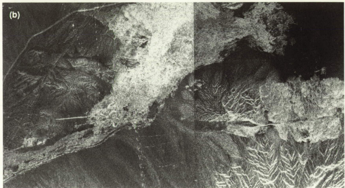
Figure 28. Pisgah Lava Field: (a) geologic map (modified from Wise, 1966, and Dellwig and Moore, 1966); (b) mosaic of two SAR L-band, HH-polarized images obtained by a NASA/JPL airborne radar system in 1985; (c) Seasat image. On the Seasat image, the bright linear feature northeast of the Pisgah Lava Field is a railroad track and the linear arrangements of bright point returns represent power lines that cross the area.
