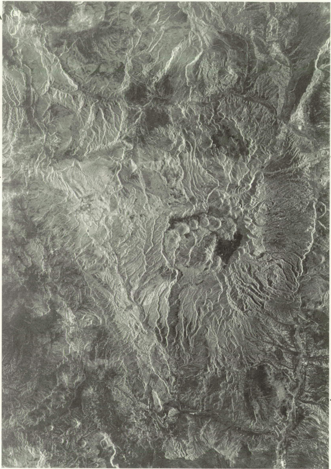
Figure 30. Jemez Mountains volcanic complex in the Rio Grande Rift, New Mexico: (a) Seasat mosaic of the region. The megamorphology of Valles Caldera surrounded by a shield-like apron of pyroclastic deposits is visible in the image. (b) Generalized map of volcanic units (modified from Ross et al., 1961). The extent of this map is indicated at the margins of the image.
