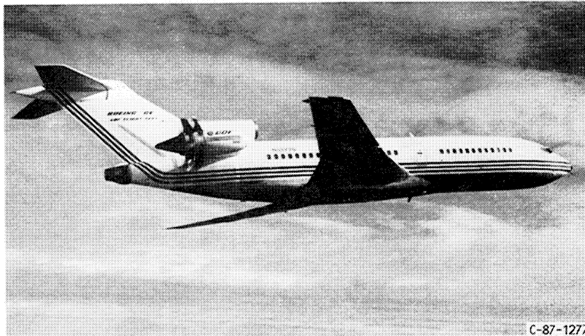
FIGURE 22. - UNDUCTED FAN (UDF) ENGINE ON THE 727 AIRCRAFT.
