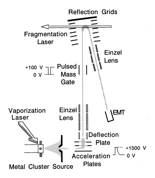
Figure 1. The reflectron mass spectrometer system used for mass selection of cluster particles followed by photodissociation spectroscopy.
