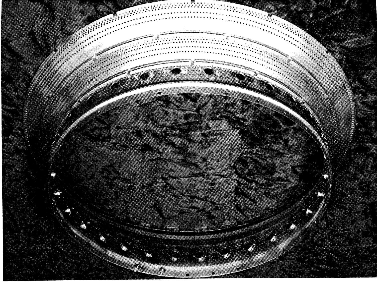
Figure 31. Combustor Inner Support Liner.
