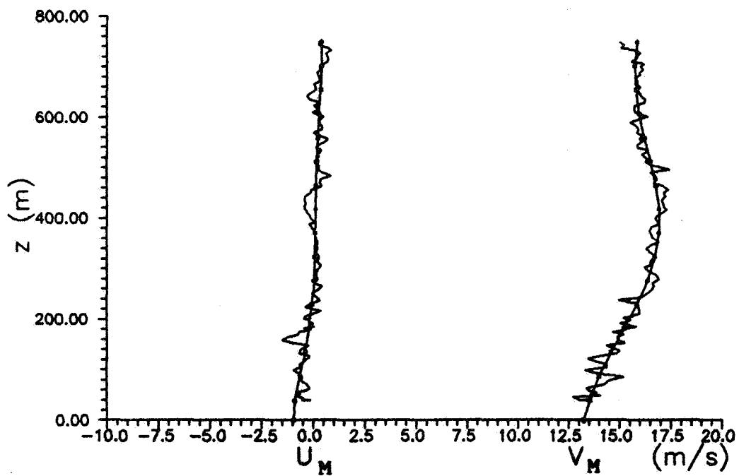
Figure 1. Cross-roll  $U_M$  and along-roll  $V_M$  wind profiles (jagged curves) measured by the NCAR Electra in the stratocumulus region on 7 July 1987 (Flight 5) between 2154:43 and 2156:49 UTC. The cross-roll, or  $x$ -, direction is  $65^\circ$  (~ENE), so that negative values correspond to winds having directions less than  $335^\circ$ . The representation of the data by the model is shown by the smooth curves.
