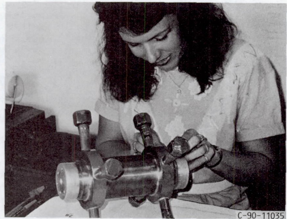
FIGURE 9. - PHOTOGRAPH OF TUBE ASSEMBLY WITH PREFABRICATED MANIFOLD INSERTS INSTALLED.
