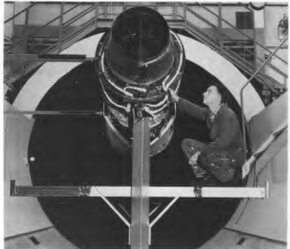
Pratt & Whitney's dual spool turbojet engine (JT3/P57) in the Altitude Wind Tunnel for nozzle studies as part of the NACA's aircraft noise suppression research, 1957.
