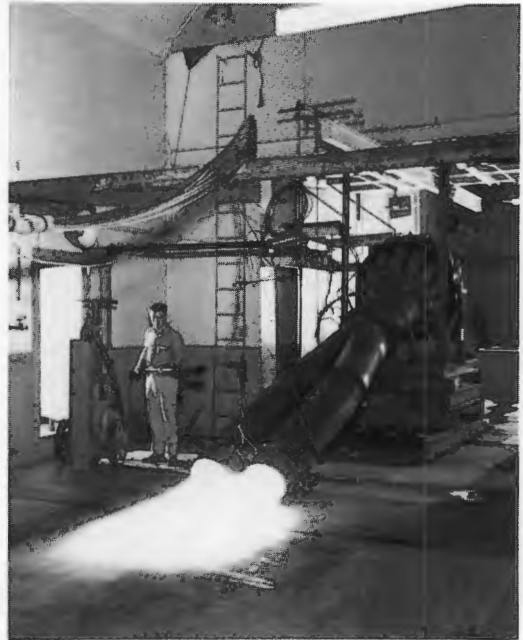
To develop afterburners required full-scale engine testing. Here a system consisting of twin exhausts is tried on General Electric's I-40, 1949.
