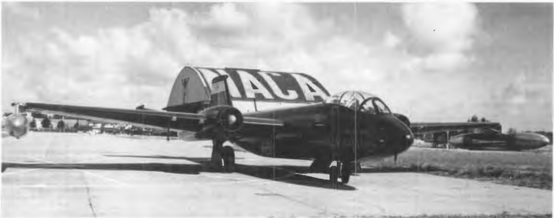
A B-57 aircraft had one engine fueled with liquid hydrogen.
