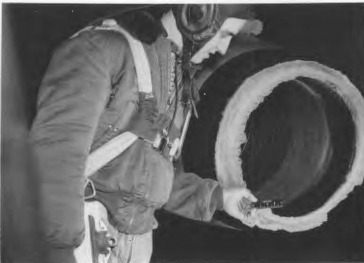
A NACA pilot measures ice on a turbojet engine's inlet. Until 1950 flight into icing clouds provided more reliable data than tests in the Icing Research Tunnel.
