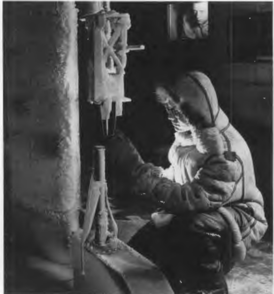
Two instruments to measure icing rates during flight through an icing cloud are calibrated in the Icing Research Tunnel. The lower device is Langmuir's rotating multi-cylinder. The upper u-tube device is the NACA pressure-type icing meter used to gather statistics on the duration and severity of icing encounters in the early 1950s.
