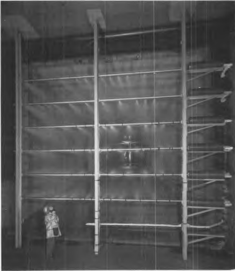
Vernon Gray investigates the new spray system, completed in 1950, for the Icing Research Tunnel.
