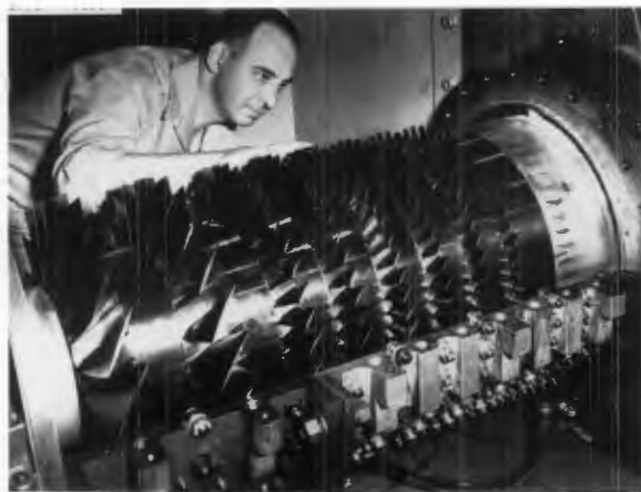
The Jacobs-Wasielewski eight-stage axial compressor perfected in the 1950s.
