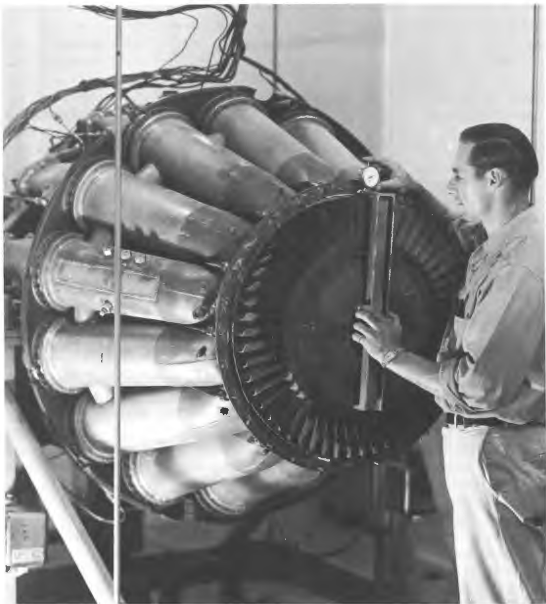
A technician uses a micrometer to determine possible distortion of the turbine blades of General Electric's I-40 turbojet engine. The ring of combustor cans, immediately behind the turbine, was Whittle's solution to the combustion problem.
