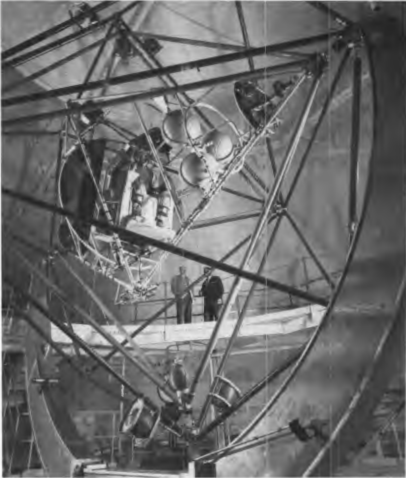
The gimbal rig at Lewis was used to teach Mercury astronauts how to bring a capsule tumbling in space under control.
