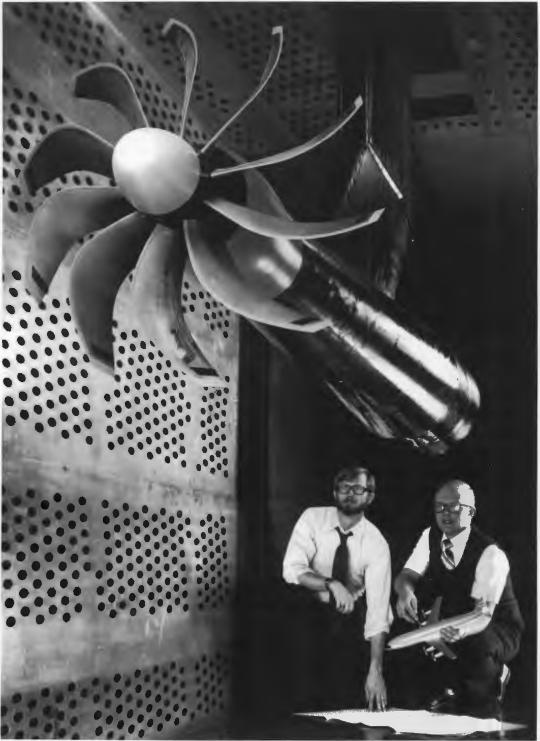
Testing the advanced turboprop. A team from Lewis won the Robert J. Collier Trophy for an outstanding contribution to aeronautics in 1987 for research begun in response to the energy crisis.
