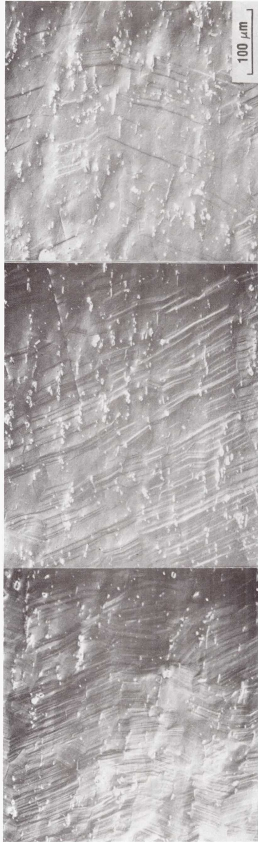
Figure 29. Surface deformation characteristics in the Al 66 Ti 25 Mn 9 bend specimen tested at 723K: (a) compression side and (b) tension side.
