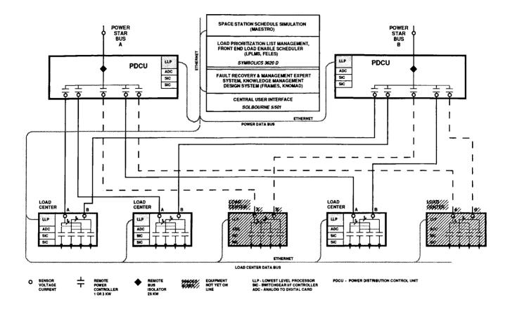
Figure 1 -- SSM/PMAD Breadboard Topology
