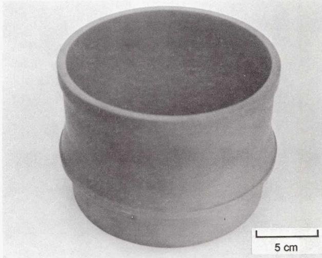
Figure 1.—View of the silicon nitride combustor.
