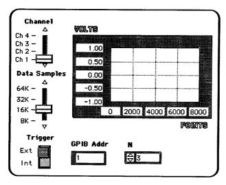
Figure 16. Waveform Analyzer VI Front Panel.
