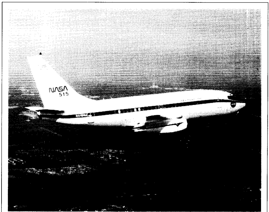
B-737 with flaps instrumented for high-lift research.
