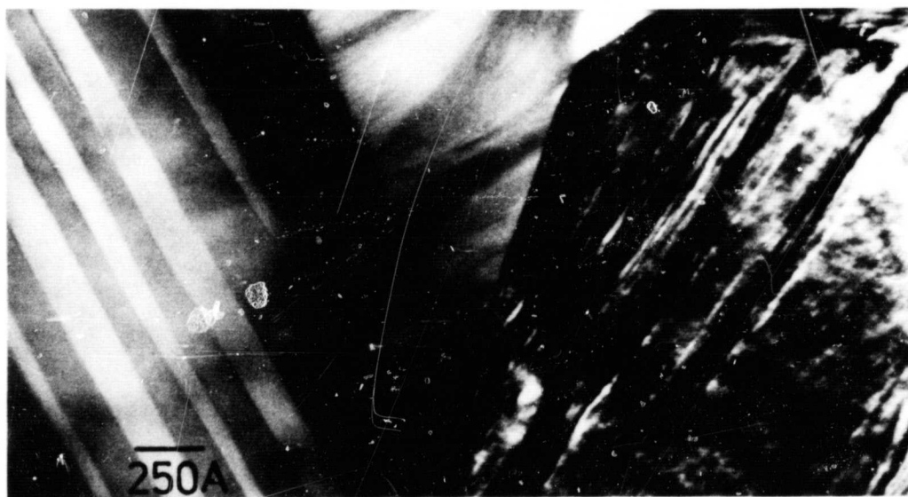
Fig 6 Edge-on (left) and inclined (right) ferroelectric domains in tetragonal PZT
