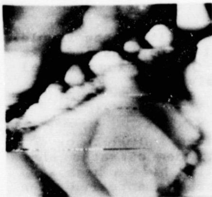
Fig. 1. Constant current image of the ZnO(0001) face. Steps are visible which form (1010) and (1120) faces. The image is 771 Å X 771 Å and was acquired at -1.5 V sample bias and 0.3 nA. The vertical resolution is 36 Å from black to white.
