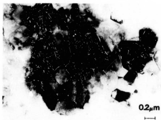
Figure 1. Transmission electron micrograph of Y-TZP (2.75 mol% Y 2 O 3 , grain size = 0.35μm).
