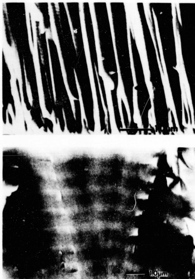
Figure 2. Scanning electron micrographs of modulated Tl_aPb_bO_c/Tl_dPb_eO_f films. Micrographs are low (top) and higher (bottom) magnifications of a cross-sectional view of a fractured film. Film was deposited by cycling electrode between 0.05 mA and 5 mA in a solution of 0.005 M TlNO_3 and 0.1 M Pb(NO_3)_2 in 5 M NaOH. Layer thicknesses are intentionally quite thick ( \sim 0.5 \mu m ) so that SEM imaging is possible.
