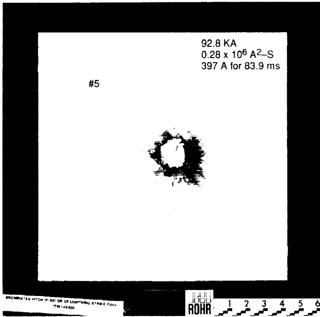
Figure 6.—Lightning strike damage on a painted P-55 pitch-based carbon fiber/epoxy composite.
