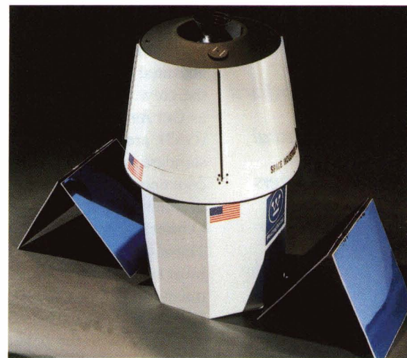
A Westinghouse official displays a model of the COMET (Commercial Experiment Transporter) service module, a key element of a new system that will enable long duration commercial space experimentation and allow recovery of some payloads for analysis on Earth; the system is shown in closeup below.
