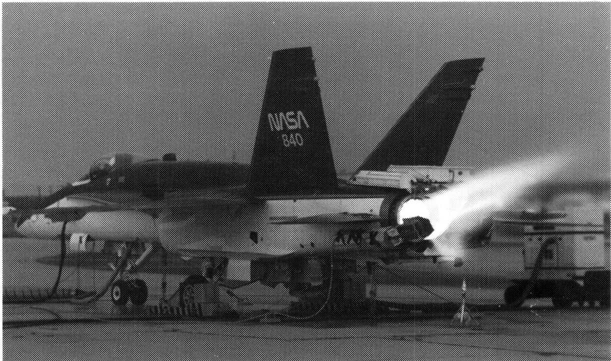
Figure 4. The F/A-18 high alpha research vehicle during single-engine thrust vectoring testing with maximum afterburner, vane 1 = -10^\circ , and vanes 2 and 3 = 20^\circ .
