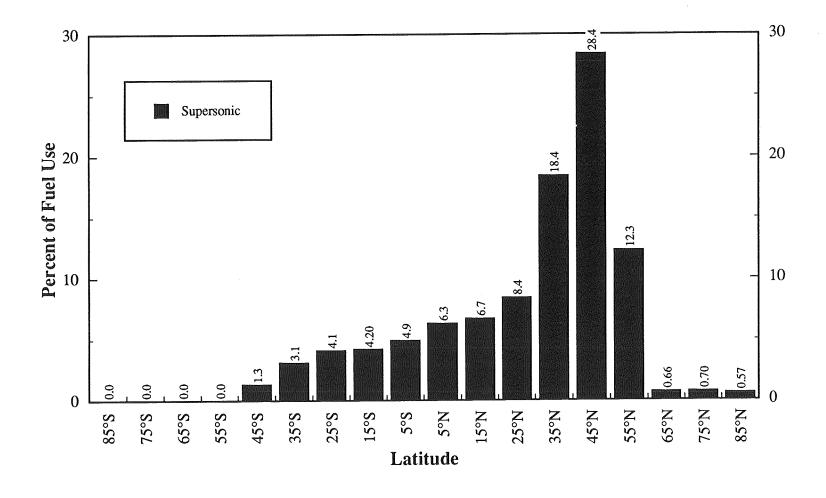
Figure 1. Latitudinal distribution of cruise fuel use for the supersonic fleet, showing the percentage of total fuel use at each latitude.
