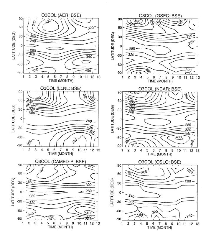
Figure 4. Calculated column abundances of  $O_3$  (Dobson units) for the baseline case (BSE) from the different models.
