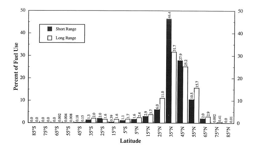
**Figure 2.** Latitudinal distribution of fuel use for the subsonic fleet at two cruise altitudes, showing the percentage of total fuel use at each latitude.
