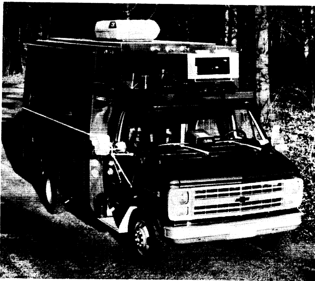
Figure 3-14 The NavLab is a testbed vehicle capable of autonomous off-road navigation.
