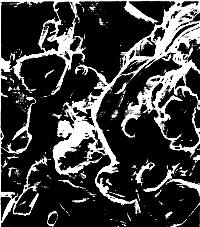
Figure 8. When superconductors were stacked for firing, the lower one showed glitter so we took a look at a) 500X SEM, and b) 1500X SEM. Note the planes within the crystals.
