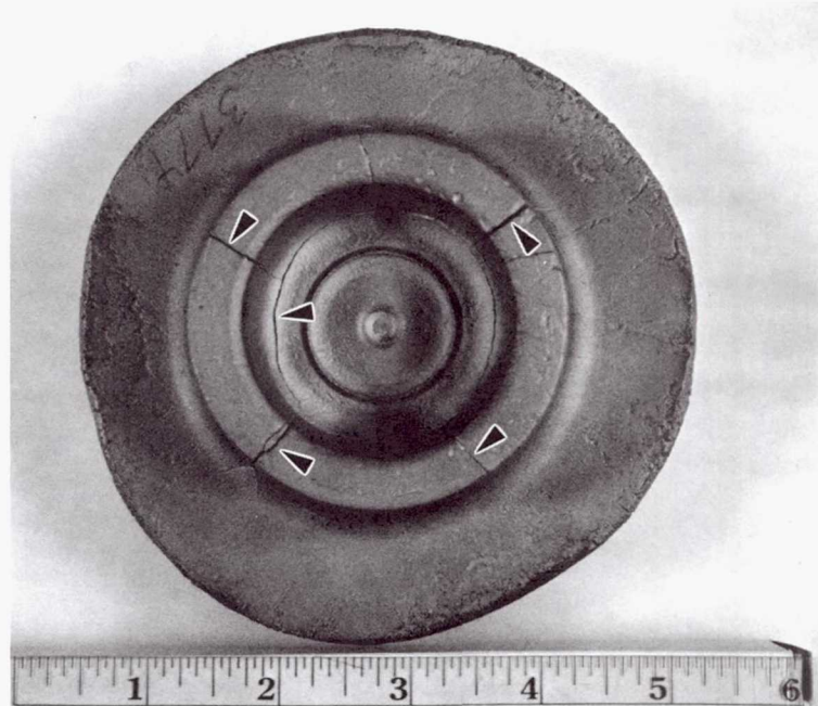
Figure 49. A shape forging of \text{Al}_{66}\text{Ti}_{25}\text{Mn}_9 : (a) top, and (b) bottom view. (Arrows in (b) indicate cracking due to CTE mismatch between the Mo punch and the part during cooling, resulting from the inability to separate the part from the punch immediately after forging).
