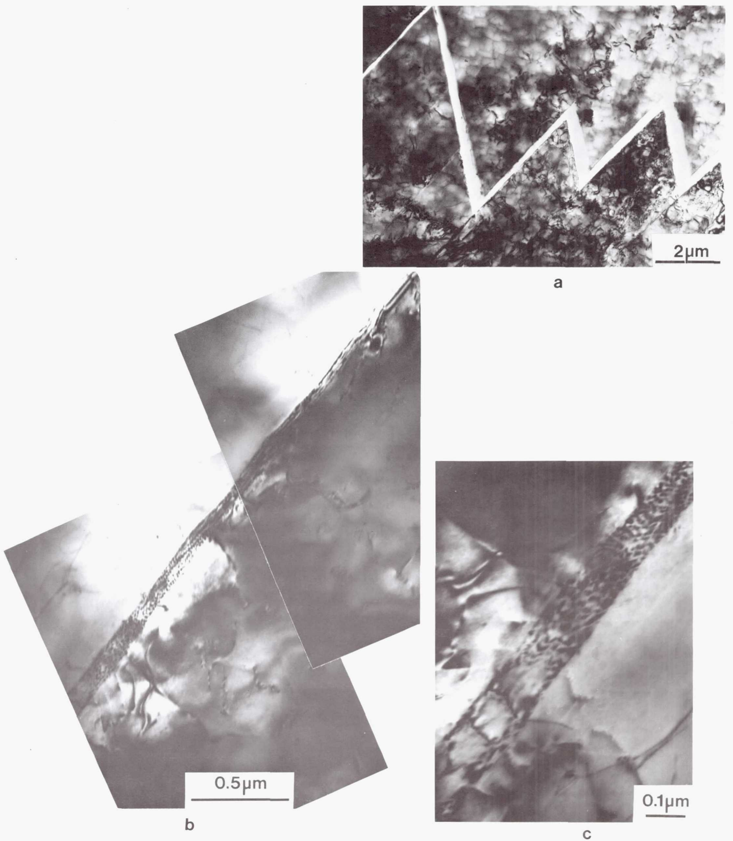
Figure 13. A crack induced at room temperature in a thin foil of the tensile specimen deformed to 18.7% at 1073K: (a) saw-tooth appearance associated with slip band formation ahead of the crack, (b,c) closely spaced dislocations lying in the slip band.
