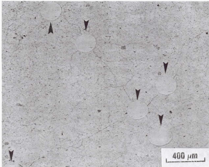
Figure 47. Fine cracks in the \text{Al}_{66}\text{Ti}_{25}\text{Cr}_9 matrix, connecting closely space W fibers (representative of ~7-8 vol.%) in the as-hot pressed condition.
