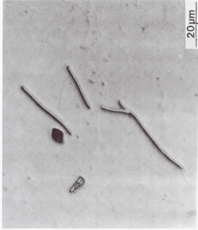
Figure 11. Optical micrographs of polished and etched cross sections obtained from the gage section (a,b) and the buttonhead grip section (c,d) of the tensile specimen deformed to 18.7% elongation at 1073K: (a) serrated grain boundaries, (b) precipitate failure, (c) undeformed grain boundaries and (d) absence of precipitate cracking.
