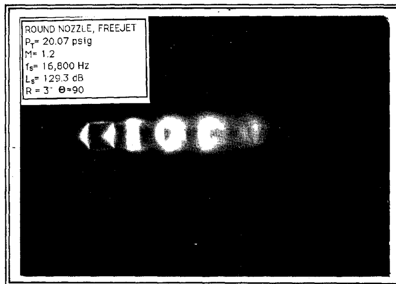
Figure 2.22 Laser schlieren flow visualization.
