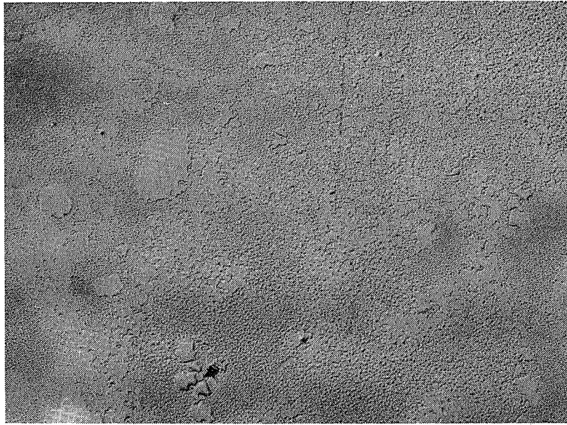
Figure 7. Photograph of LiF window, front surface, 40X.
