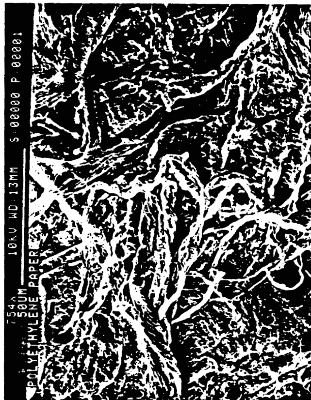
POLYETHYLENE PAPER - AS RECEIVED - 754X
