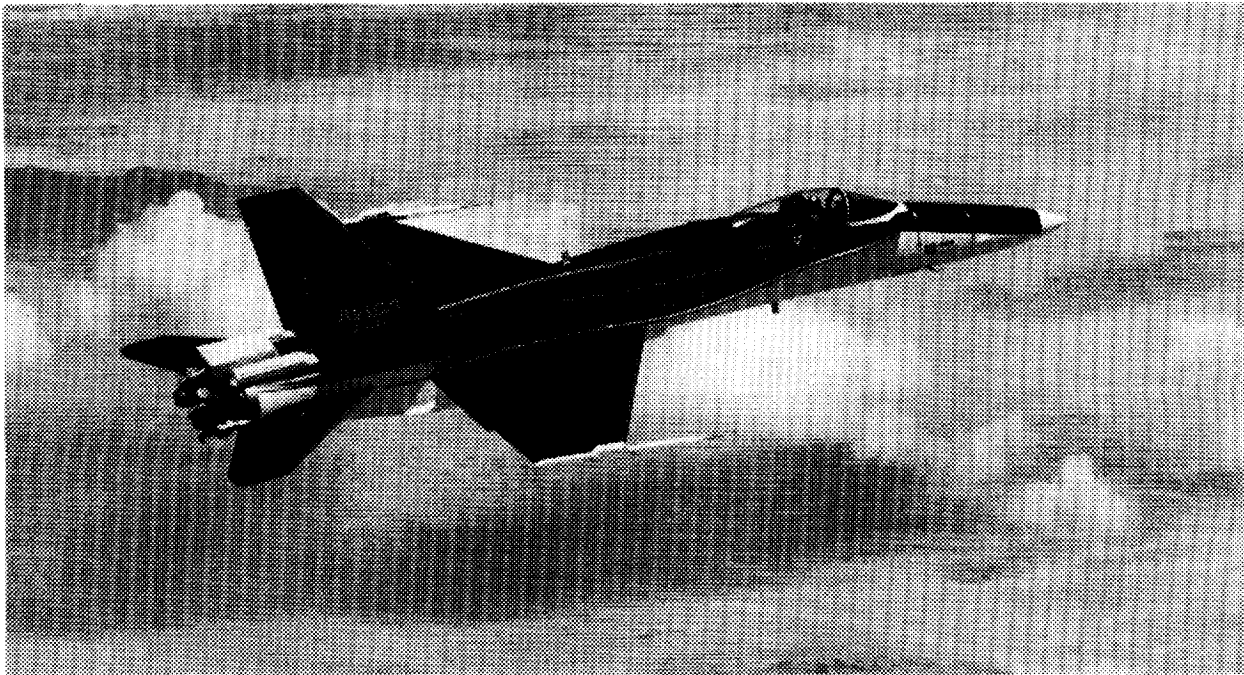
Figure 26. The thrust vectoring system installed on the HARV. A spin recovery parachute is mounted in the box between the upper vane actuator fairings.
