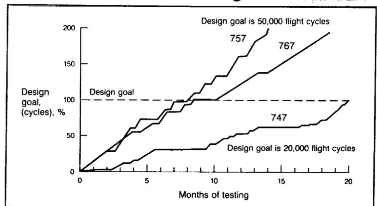
time, without any down-time caused by structural fatigue cracking. The Structures Durability Program goal of reducing up to 85% of detail design problem areas was far exceeded.
