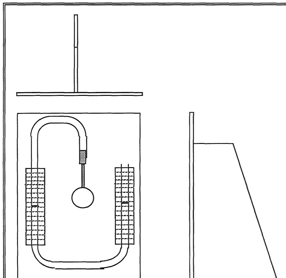
Figure 1: A sketch of the U-tube manometer. Details of the tube are omitted from the top and side views. The stand that holds the manometer vertical is hinged for storage. The vinyl tube is attached to the masonite background with soft wire. The needle must be placed far enough away from the backplate that the bubble will not touch the plate.
