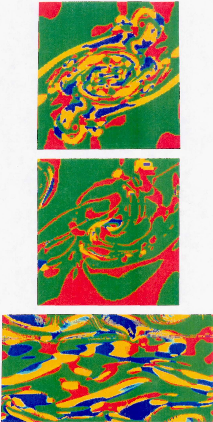
FIGURE 5. Maps of the local flow topology in two planes: (a) vertical rib plane, incompressible case, (b) vertical in-between plane, incompressible case, (c) horizontal plane at the middle of the layer, compressible case. See Figure 2 for color code.
