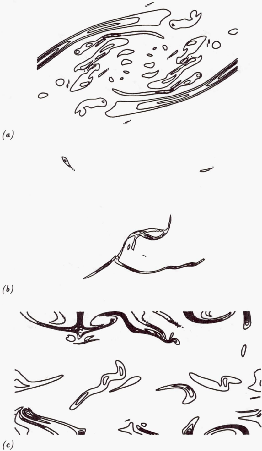
FIGURE 3. Maps of the enstrophy field in two planes: (a) vertical rib plane, incompressible case, (b) vertical in-between plane, incompressible case, (c) horizontal plane at the middle of the layer, compressible case.
