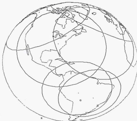
Coverage with 2 Planes @ 6 Satellites/Plane
