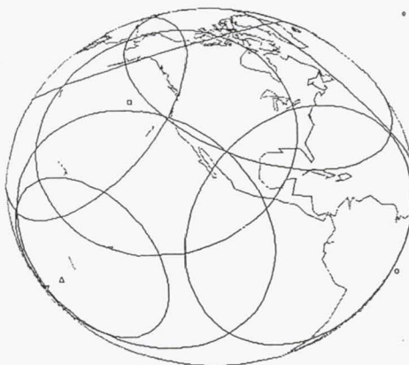
Coverage of 2 Planes x 6 Satellites Constellation with 6 Additional Equatorial Satellites
