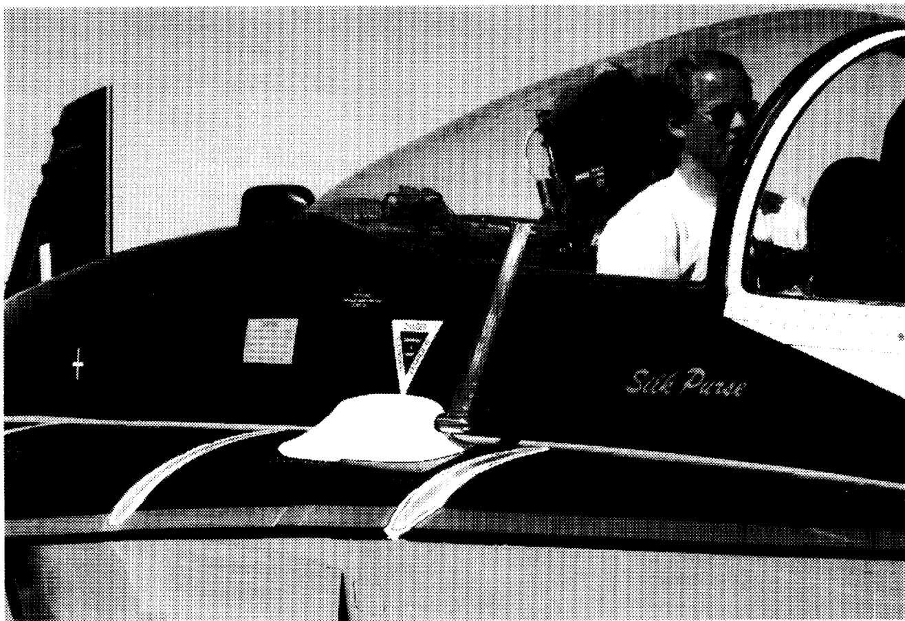
Figure 3. LEX survey rake located on the upper surface of the right LEX with the probe tips located at F.S. 253.
