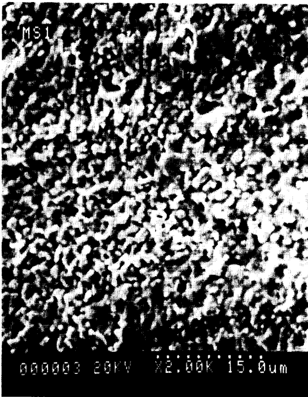
Figure 3.2.2-3. Uncoated NASA-Z Cylinder After Oxidation and Reduction Test Cycle-26 Slot Area (1.8% Strain)
