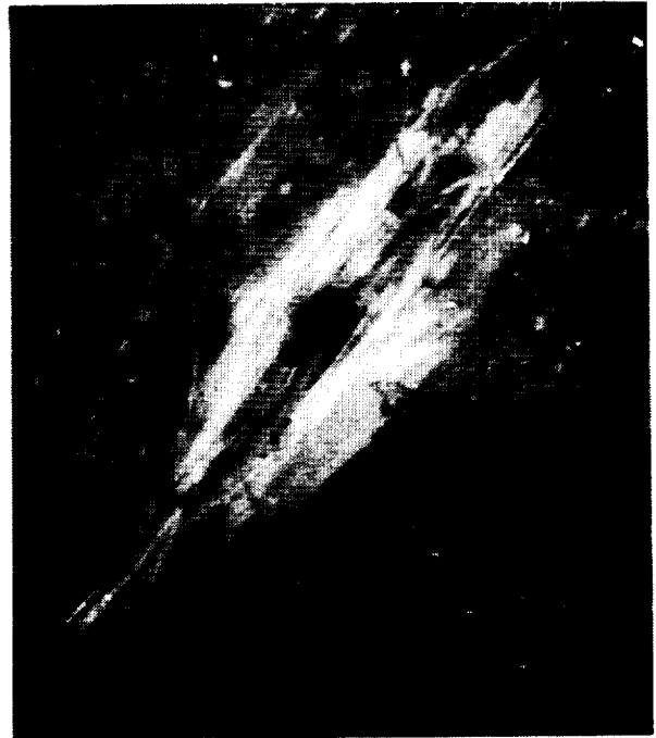
Fig. 19 Micrometeoroid/Debris Impact Damage (x100) on Kevlar®/Epoxy Tube [SP-328, (\pm 45^\circ)_4S ]
