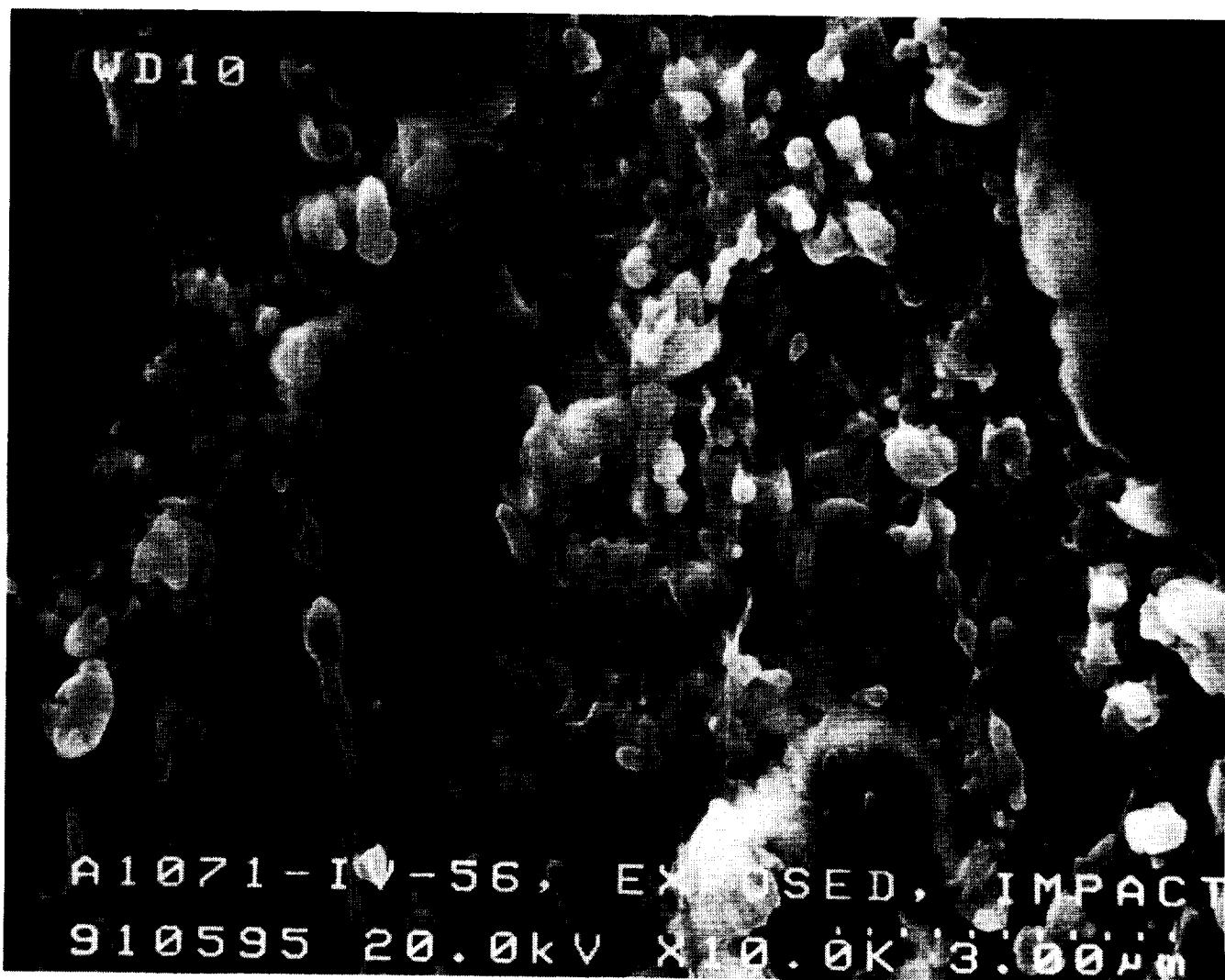
Figure 4. Scanning Electron Microscope View of Sample Coated With Aluminum Produced From Debris Impact.
