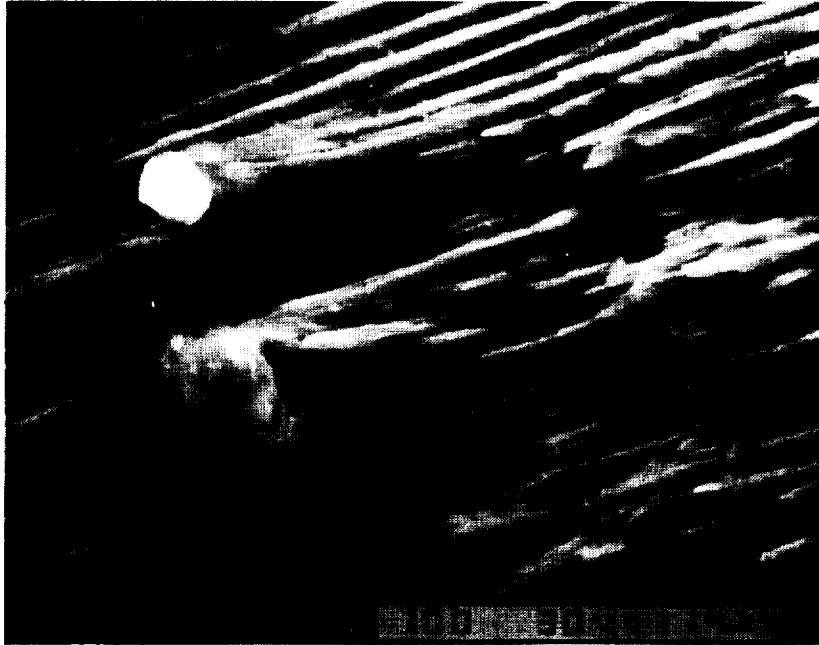
Fig. 8 SEM Photograph of Surface Morphology on Exposed Graphite/Epoxy Tube [934/T300, (90°) 4S ]
