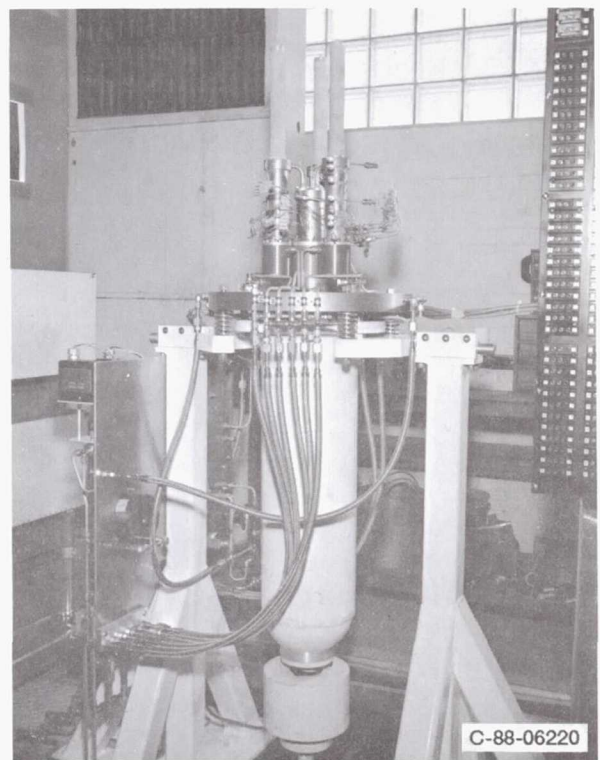
Figure 14.—HP-1000 heat pipe Stirling engine.
