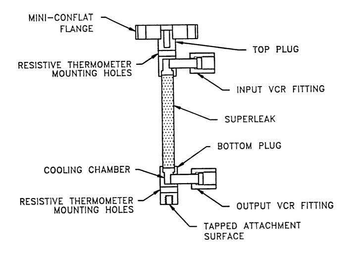
Figure 18 Scale Drawing of Finalized ACE, Inc. Vortex Cooler Design
