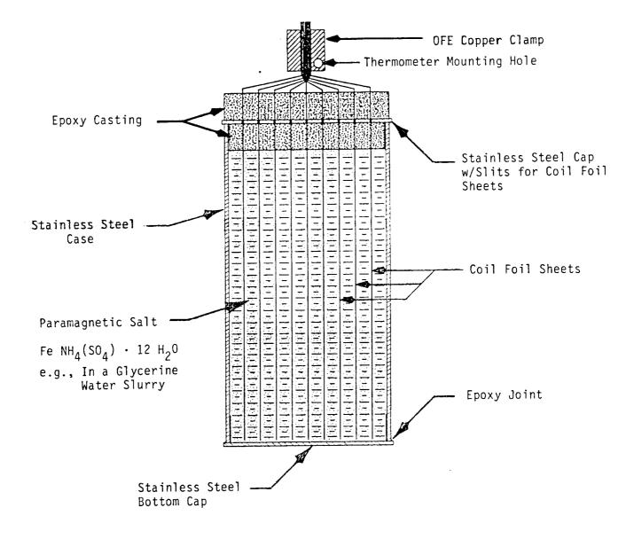
Figure 27 Schematic Representation of ADR Salt Pill
