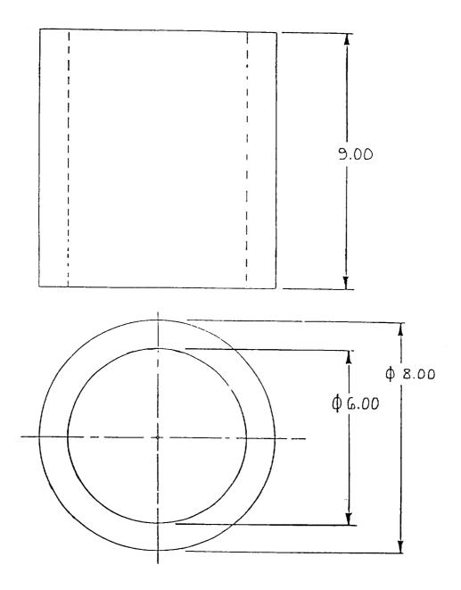
Figure 31 Side View of Magnetic Shield
