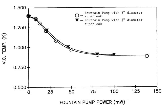
Figure 17 Vortex Cooler temperature as a function of Fountain Pump power for two different Fountain Pump Superleak diameters.
