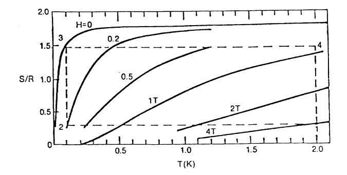
Figure 1 Entropy versus Temperature Chart for Ferric Ammonium Alum. From Castles (1980)
