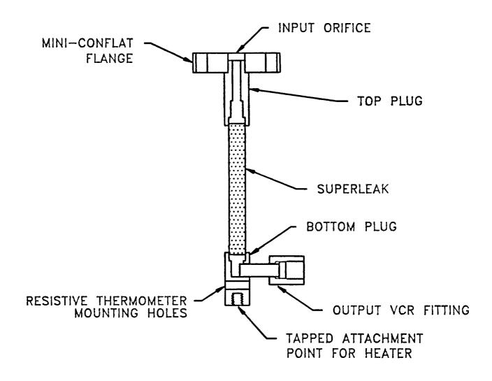
Figure 19 Scale Drawing of Finalized ACE, Inc. Fountain Pump
