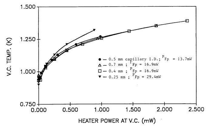
Figure 15 Vortex Cooler Temperature as a function of Heat Load applied to the Vortex Cooler for various Vortex Cooler Exit Capillary Sizes. The Fountain Pump Power Fp for each curve has been adjusted to minimize the temperature of the Vortex Cooler under zero Heat Load.
