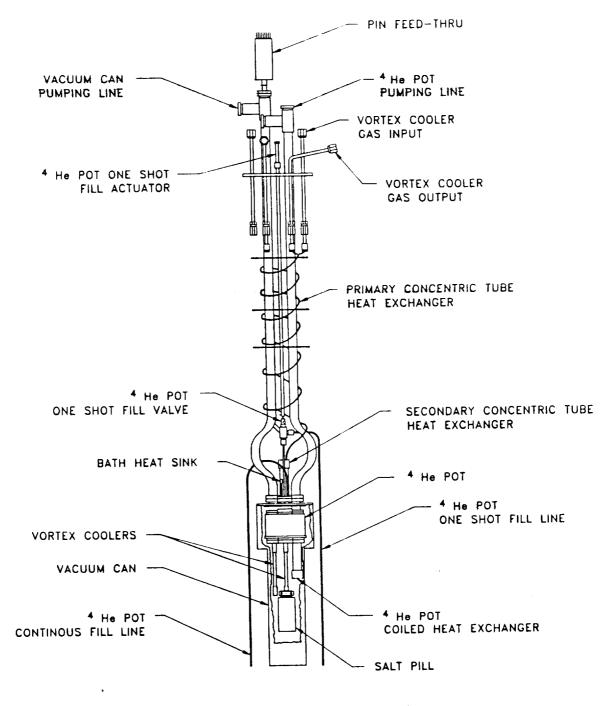
Figure 4 ADR Cryostat Configuration
