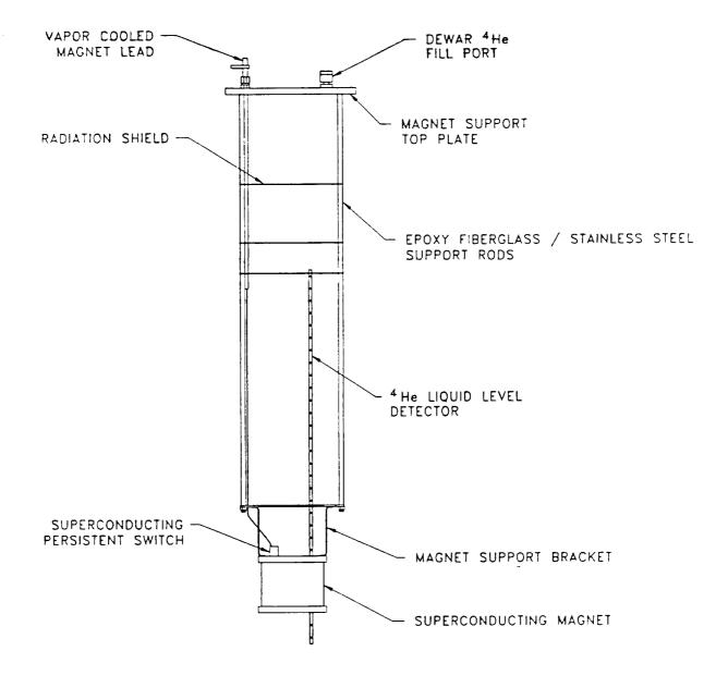
Figure 7 Superconducting Magnet Support
