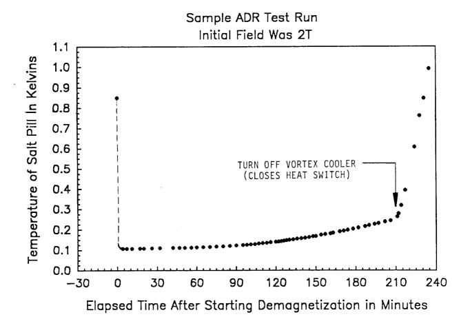
Figure 29 Cooling curve for the ACE, Inc. Adiabatic Demagnetization Refrigerator
