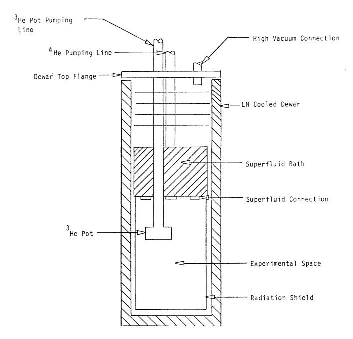
Figure 9 Auxillary Test Facility
