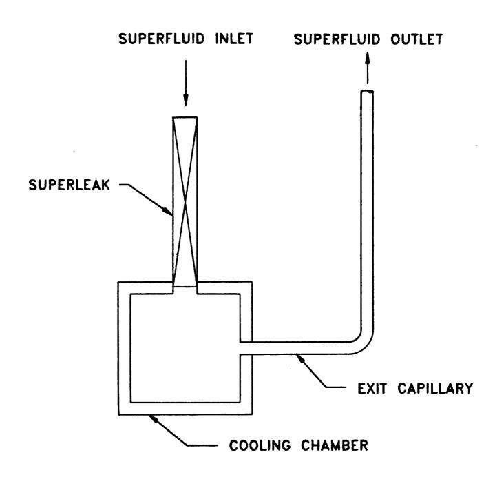
Figure 11 Schematic Representation of a Vortex Cooler
