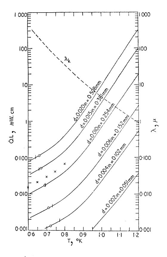
Figure 13 Heat Leak Along Superfluid Filled Capillaries as a Function of Temperature for (0.6 K < T < 1.2 K). The data is shown for different capillary diameters.
