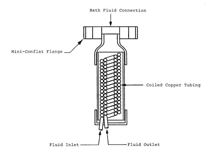
Figure 20 4He Pot Coiled Heat Exchanger
