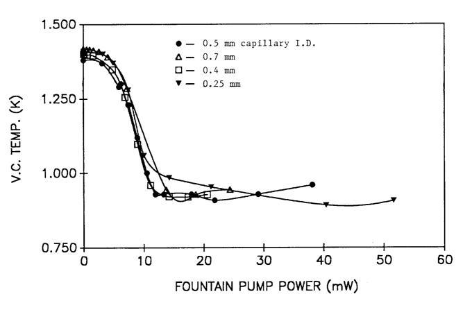
Figure 14 Vortex Cooler Temperature as a function of Fountain Pump Power for various diameter Vortex Cooler Exit Capillaries.
