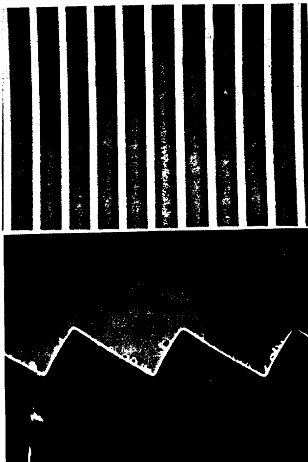
Fig. 1. Scanning electron micrographs of blazed Echelle gratings etched photoelectrochemically in the (100)-18° surface of n-GaAs. Groove spacing is 20 \mu\text{m} .
