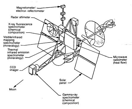
Several geophysical instruments—a combination magnetometer and electron reflectometer, a radar (or laser) altimeter, and possibly a microwave radiometer—would gather important geophysical data.
