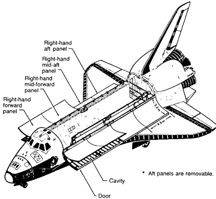
b. The panels have a heat rejection capacity of 5480 kJ/hr (5400 Btu/hr) during ascent through the atmosphere with the doors closed and 23 kJ/hr (21.5 Btu/hr) during orbital operations with the doors open.
