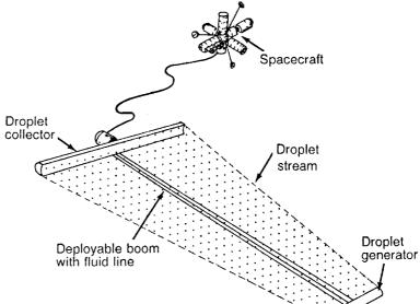
It was demonstrated some time ago that liquid droplets with very small diameters (about 100 micrometers) are easily manufactured and offer a power-to-mass advantage over solid surface radiators of between 10 and 100. In effect, large, very thin radiator sheets can be produced by the proper dispersion of the droplets. This system offers the potential of being developed into an ultralightweight radiator that, since the liquid can be stored in bulk, is also very compact.
