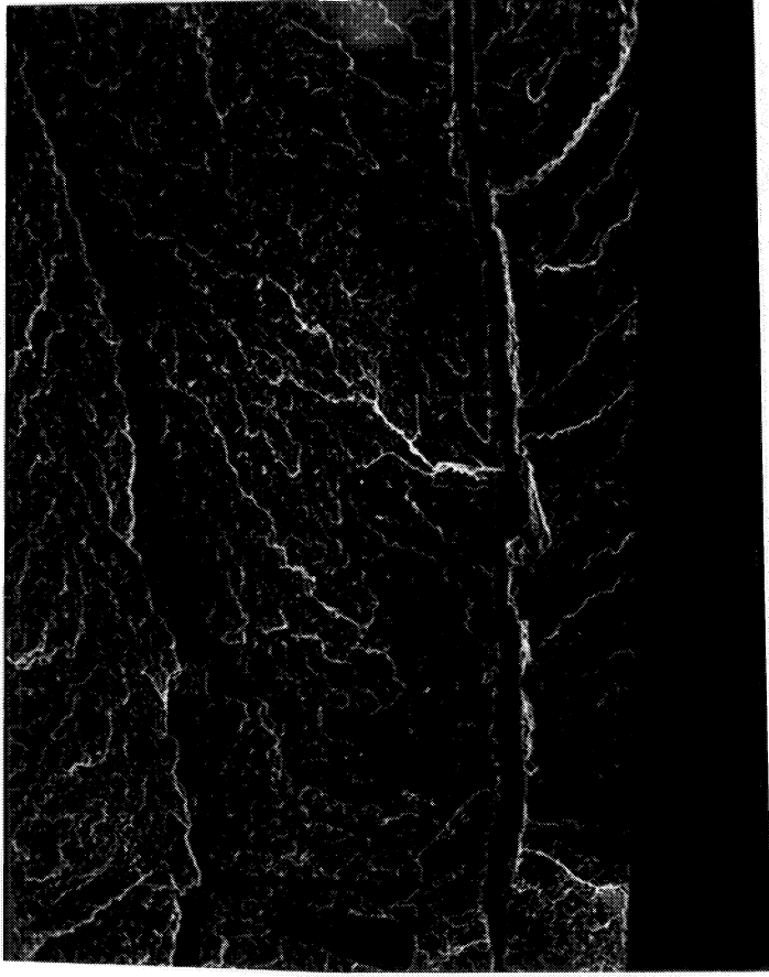
↑ fig 10 cracks in BF062 fractured in hydrogen
