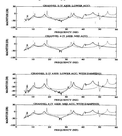
In the second test for both approaches, a "modal" damping matrix was calculated using the measured eigenvalue  $(2\zeta\omega_n)$  and the original eigenvectors. With the original eigenvectors mass orthogonalized, a physical damping matrix was approximated by the following:
