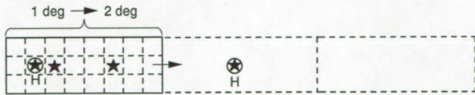
Fig. 5. Star observations with a scanning telescope and CCD detector. (Hipparcos stars are marked with an H.)
