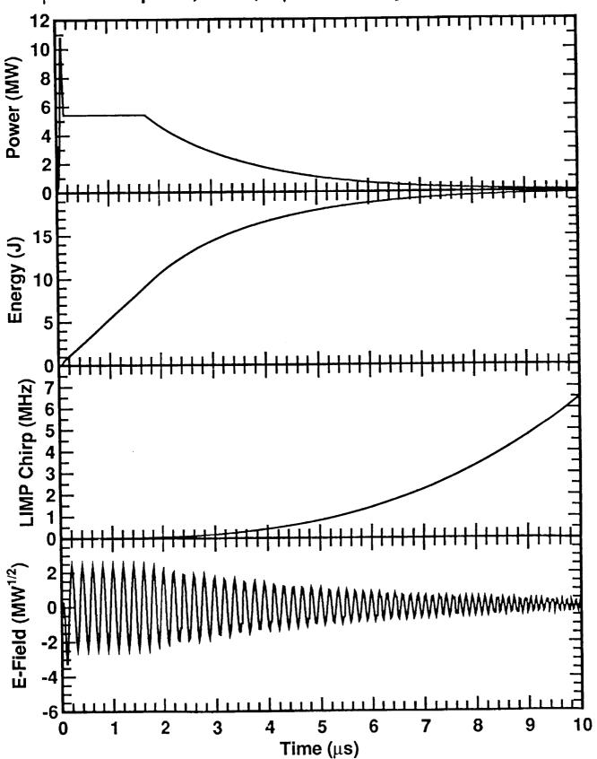
3.1  $\mu s$  FWHM pulse, GSS , 4  $\mu s$  tail decay and frequency chirp
