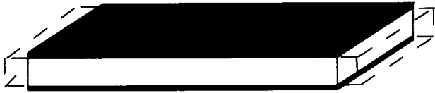
Figure 3. Lengthening effect ( d_{31}, d_{32} effect).
