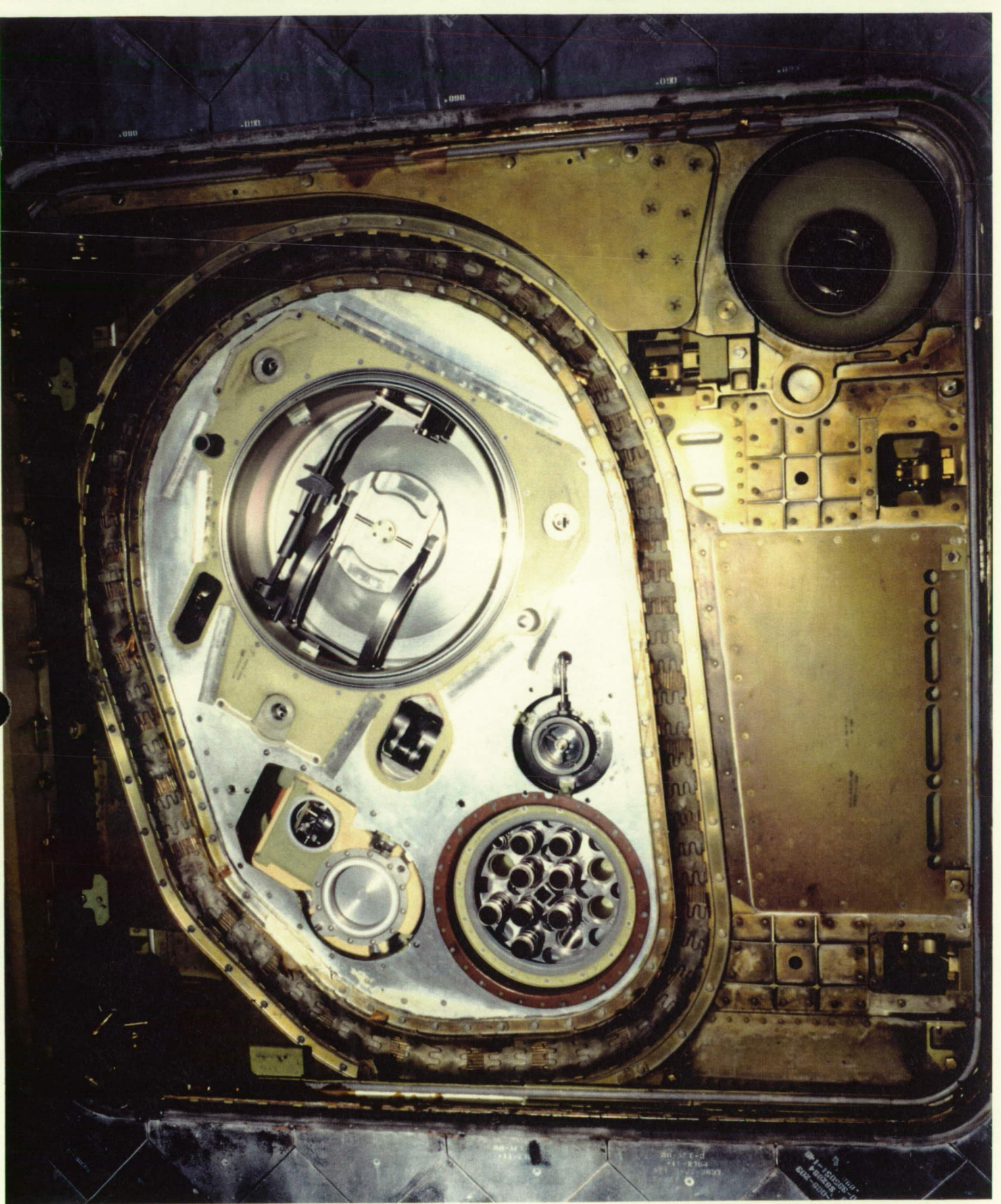
Overall view of the LH2 ET/ORB umbilical. All separation ordnance devices functioned properly. No flight hardware was found on the runway below the umbilical when the ET door was opened.
