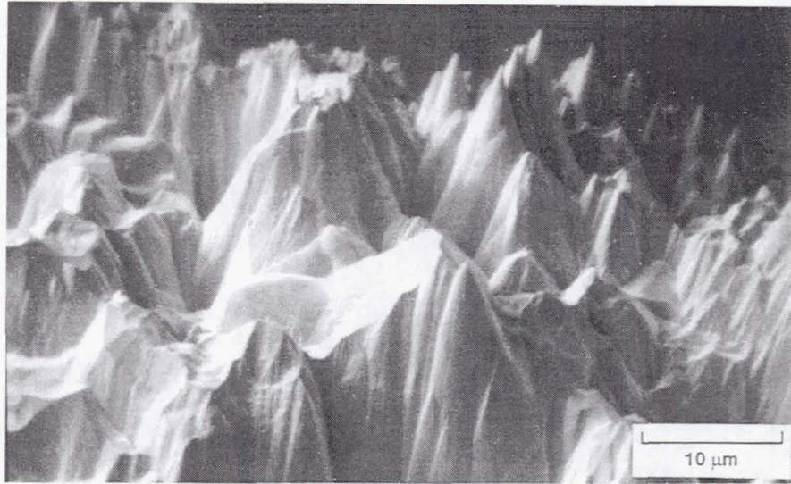
(c) Severe cone formation visible after 13 hr of sputtering.
