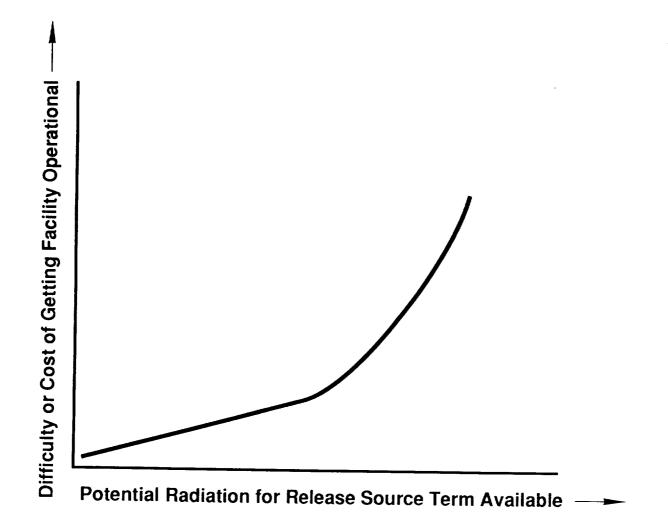
Figure 4-1. Cost Profile of Reactor/Engine Test Facility vs Source Term Available for Release
