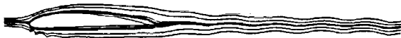
Figure 16: Superposition of the steady solution and higher mode disturbance for the NACA 4412 airfoil, Re = 300
